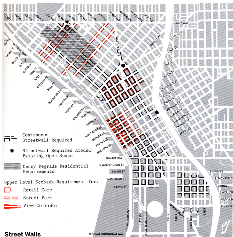
図 7-3-5 土地利用・交通プラン素案：街路壁・上階壁面後退 (Land Use and Transportation Project, City of Seattle (1983) “Draft Land Use and Transportation Plan for Downtown Seattle”, p.65)
